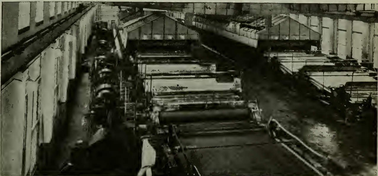
The "wet" end of two Fourdrinier paper machines. In the foreground is the shaking wire on to which the pulp flows. The right-hand machine shows the blanket which takes the pulp sheet from the wire.
